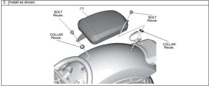
3. Install the motorcycle's parts in the reverse order of removal.
